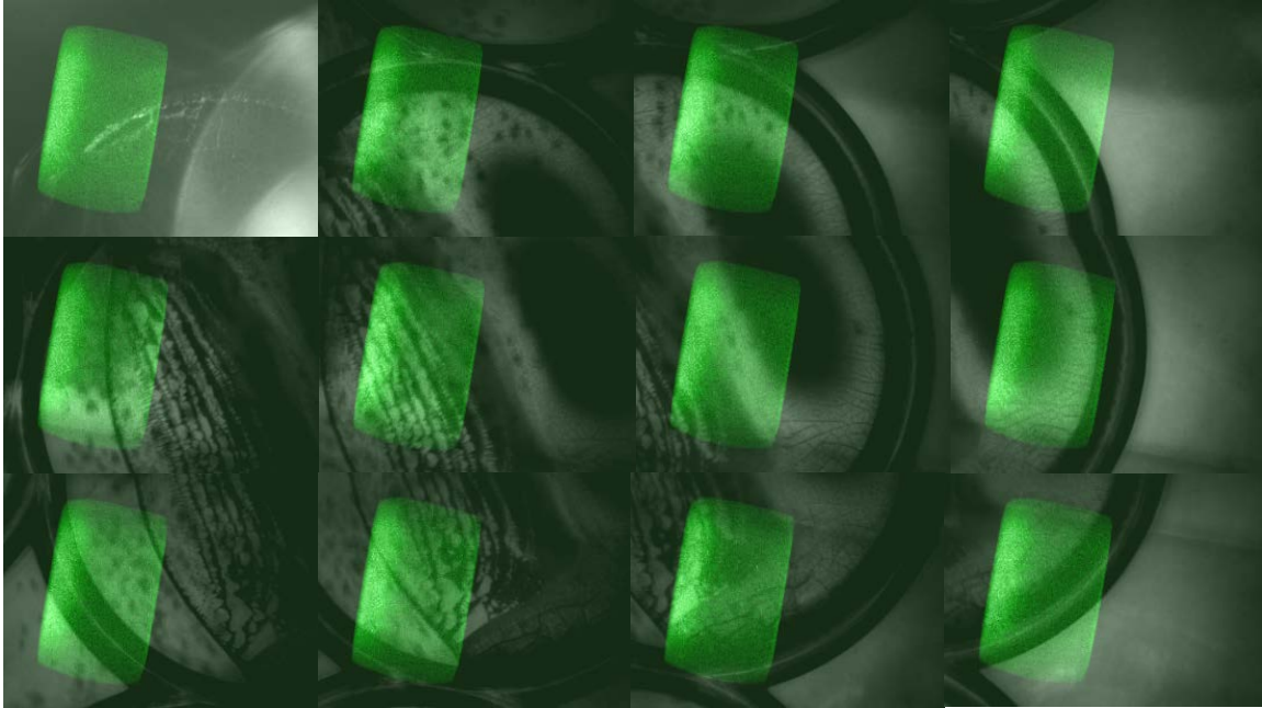
Figure 14. The QASPR-3 proton beam was able to hit the total area each well by firing shots in a grid pattern based on the area of the beam. Top Row: Shots 1-4; Center Row: Shots 5-8; Bottom Row: Shots 9-12.
